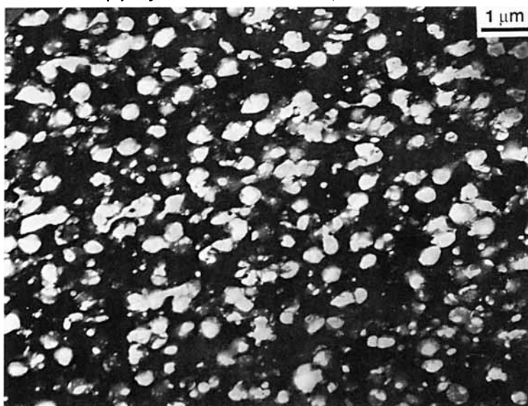
Figure 10 TEM photomicrograph for nylon 6/ABS/IA-250-C (45/45/10) blend prepared in 25.4 mm single-screw extruder stained with (a) \text{OsO}_4 and (b) PTA.
